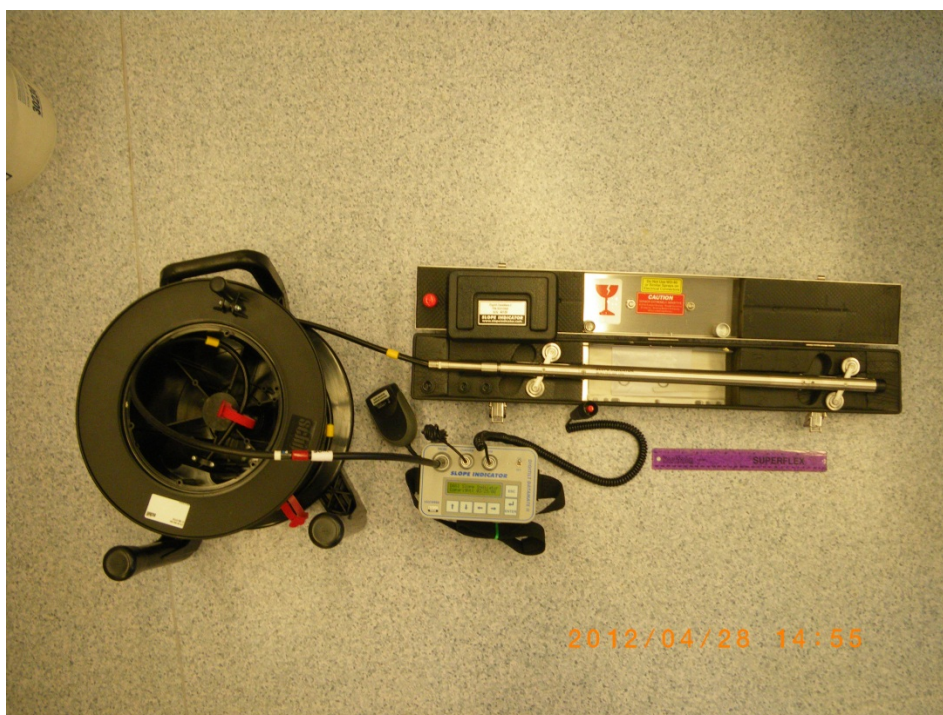
Photo 3: Slope Indicator's Digitilt Inclinerometer Probe with Digitilt DataMate II datalogger with battery charger and remote hand switch, and 30 m Digi Control Cable on a 50 m Capacity Digitilt Cable Storage Reel,
